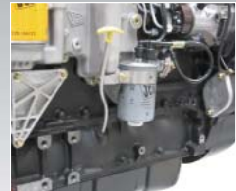
Bedplate, integrated oil cooler & second power take off
