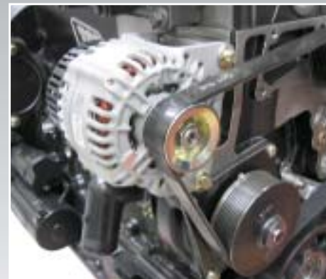
Integrated water pump & alternator mounting with poly vee drive
